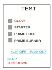
This screen features diagnostic tools to aid in the installation and testing the various turbine systems, in particular the priming of the fuel and burner.
