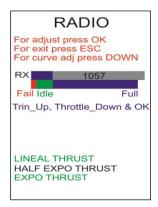
Note: For FUTABA systems you must reverse the throttle channel, Jeti and JR systems require non-reversed settings, other systems will require verification using the graphical display in the Radio Menu.
