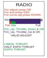
5.6.1.1 Transmitter Preparation and VerificationThe radio screen features an indication of the transmitter channel current throttle stick position by using a graphical slider display of the Pulse Width value; the actual pulse width value will also be displayed numerically in milliseconds (mS). Verify that the throttle stick movement is correct from end to end and is fast. Once the transmitter has been verified, the learning process can be started for the POWERPACK / ECU.
