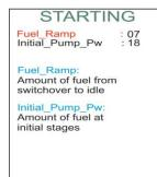
There are only two adjustable parameters in this sub-menu, "Fuel Ramp" values and "Initial Pump Pw".
