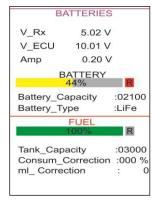
In the center of the display menu there are two settable parameters, "Battery Capacity" and "Battery Type". The selections for Battery Type are "LiFe" or "LiPo", capacity should be set to match the ECU battery.
