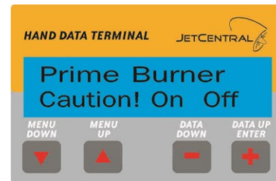
Test Prime Kerosene Burner
