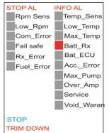
"Temp\_Sens" indicates a temperature probe failure.
