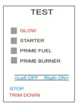
This screen features diagnostic tools to aid in the installation and testing the various turbine systems, in particular the priming of the fuel and burner lines.
