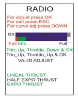
5.6.1.1 Transmitter Preparation and VerificationThe radio screen features an indication of the transmitter channel current throttle stick position by using a graphical slider display of the Pulse Width value; the actual pulse width value will also be displayed numerically in milliseconds (mS). Verify that the throttle stick movement is correct from end to end and is fast. Once the transmitter has been verified, the learning process can be started for the POWERPACK / ECU.
