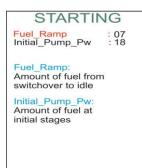
There are only two adjustable parameters in this sub-menu, "Fuel Ramp" values and "Initial Pump Pw".
