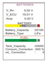
In the center of the display menu there are two settable parameters, "Battery Capacity" and "Battery Type". The selections for Battery Type are "LiFe" or "LiPo", capacity should be set to match the ECU battery.
