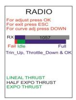
Note: For FUTABA systems you must reverse the throttle channel, Jeti and JR systems require non-reversed settings, other system will require verification using the graphical display in the Radio Menu.
