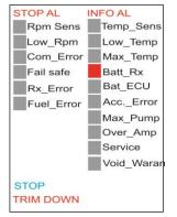
"Temp\_Sens" indicates a temperature probe failure
