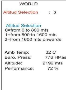
To set the local altitude enter the value corresponding to your local altitude, the values are 0 through 2, the ECU measured altitude which is displayed on the lower section of the display should be used as a reference.
