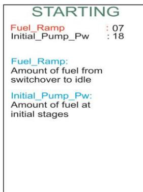
There are only two adjustable parameters in this sub-menu, “Initial pump Pw” values and “Fuel Ramp”.
