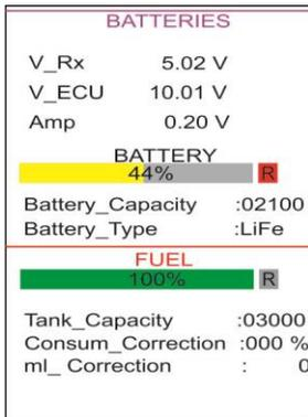
The top portion of the battery menu display indicates the RX Battery Voltage, ECU Battery Voltage and the current (in Amps) being consumed from the ECU battery.
