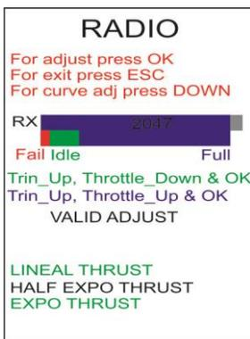
The radio screen features an indication of the transmitter channel current throttle stick position by using a graphical slider display of the Pulse Width value; the actual pulse width value will also be displayed numerically in milliseconds (mS). Verify that the throttle stick movement is correct from end to end and is fast. Once the transmitter has been verified, the learning process can be started for the POWERPACK / ECU.
