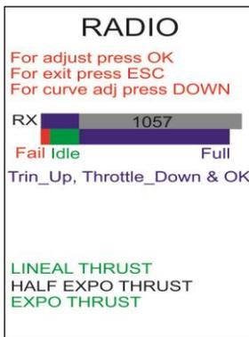
To program the throttle stick position value into the ECU select “Ok” on the HDT. Move your transmitter trim up all the way and your throttle stick down; then press “OK” on the HDT.
