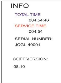
The info menu is used to display the Total Time, Service Time, Turbine Serial Number, and the Software Version of the Power/Pack ECU.
