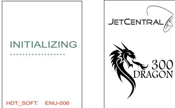
When the POWERPACK / ECU is connected to the HDT, the ECU battery is connected and the RX power is turned on, the HDT display screen will briefly display "INITIALING" with the software version of the HDT displayed across the bottom of the display, and then briefly displays the Logo of the turbine that is connected, after a few seconds the main screen will be displayed.
