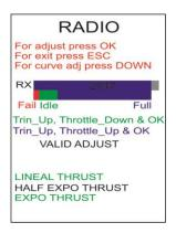
5.6.1.1 Transmitter Preparation and VerificationThe radio screen features an indication of the transmitter channel current throttle stick position by using a graphical slider display of the Pulse Width value; the actual pulse width value will also be displayed numerically in milliseconds (mS). Verify that the throttle stick movement is correct from end to end and is fast. Once the transmitter has been verified, the learning process can be started for the POWERPACK / ECU.
